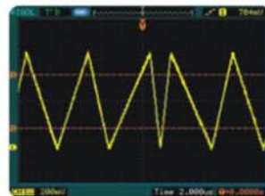
Slope Trigger Trigger by signal rise time or fall time
