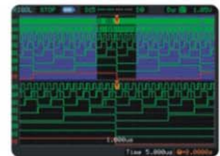
Duration Trigger Combination of Pattern Trigger and Pulse Width Trigger
