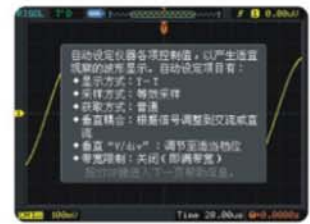
Built-in Help System Press current key for 3 seconds to enter help system
