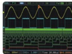
Pattern Trigger Trigger condition is the combination of level and edge
